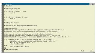
Illustration 9: Script for determining the space used on the root partition
