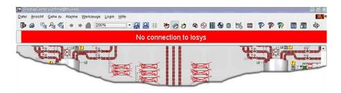
Illustration 65: Display of the system error message noiosysconnection
