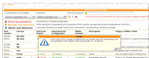
Illustration 21: Port scan with an external scan server in the APROL SDM
